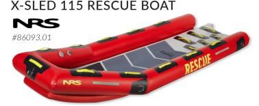
The NRS X-Sled 115 Rescue Boat gives rescuers the options needed for swiftwater, ice, low-head dam and floodwater rescues. Designed to accommodate two rescuers and one victim but can easily float 4-5 people.
