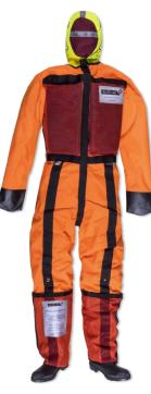
The Man Overboard Water Rescue Manikin is built to simulate an unconscious victim in the water, floating at an angle of 45 degrees with just the head and shoulders above the water. It can be made to float horizontally by simply removing the 6 foam pieces from the front chest of the coverall and adding three pieces to the pockets on each leg.
