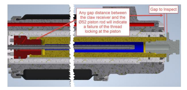
4. If gap is found  $\rightarrow$  tag ram rescue tool for repair, remove from service and contact your service provider.
