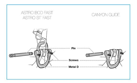
The defect is due to a poor machining process of the metal D. This can cause the pin to slide completely sideways, despite the presence of the 2 screws. This situation presents a risk of death due to strangulation or falling from a height.
